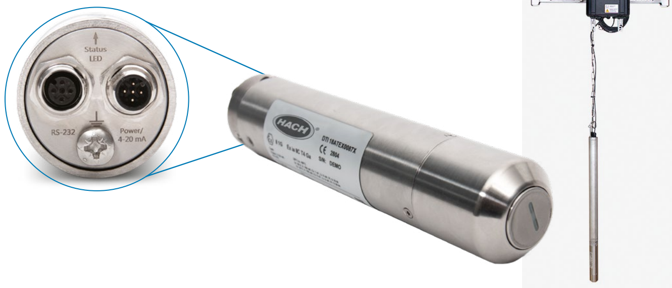
Figure 2. This compact, low-maintenance, electrochemical sensor – with stainless-steel housing, anti-fouling design, and sealed industry-standard connections (shown in callout) – provides robust performance for submerged wastewater as well as gas-phase applications. It delivers \pm 5 -percent accuracy with a detection limit of 1 percent of full range. The same sensor can report in milligrams per liter (mg/L) for liquid measurements and parts per million (ppm) for gas/air measurements. Standard bracket assemblies (inset) provide for quick and convenient mounting in typical manhole locations.
